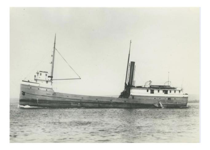
The M. T. Greene was classified as a steam barge. It served as a bulk carrier and a tow vessel.
