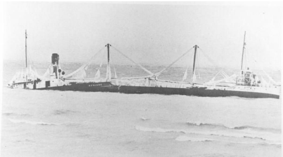
Bottom – Novadoc – Back broken and sheathed in ice aground on Lake Michigan
