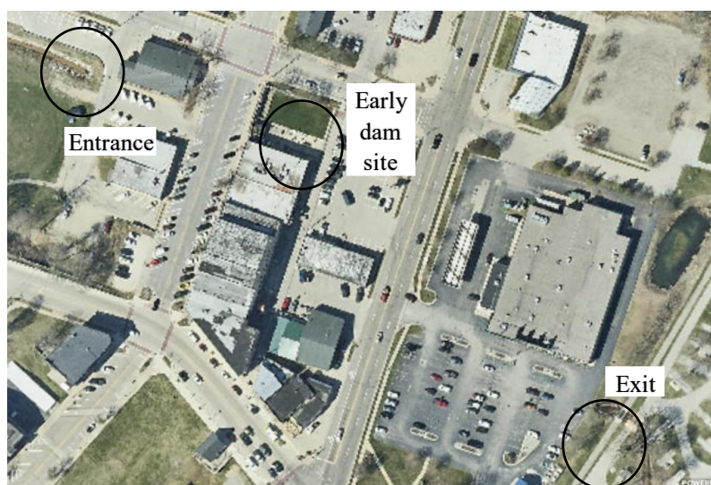
Figure 2. Buttermilk Creek piping under Montague, and early dam location
